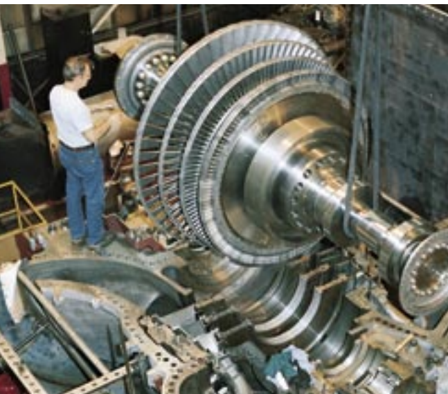
This four-stage low-pressure CAES expander has an output of 100+ MW with a 1,600°F (871°C) inlet temperature.
