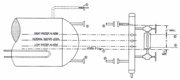
SHUTOFF VALVES BETWEEN DRUM AND COLUMN MUST BE OS&Y, OF THROUGH-FLOW DESIGN AND ORIENTATION, SHOW POSITION AS OPEN OR CLOSED, AND HAVE LOCK- OPEN CAPABILITY.
